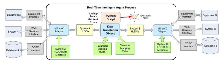
By contrast, MilramX uses the paradigm of intelligent agents which are run as separate processes in parallel on multi-core processors running the Windows operating system. In this way each intelligent agent process can monitor a one or more sources of data for changes and then make decisions, advise people, and/or communicate with other agents in near real-time.
