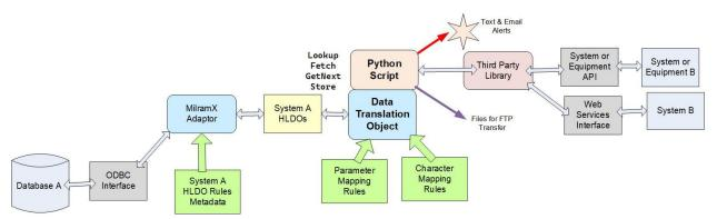
Instead of using the MilramX adaptor mechanism, MilramX DTOs can also use third party libraries to interface to external systems. This can be especially beneficial when all the work has been done by someone else to reduce the complexities of interacting with systems which have complicated interface protocols.
