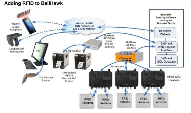
BellHawk is an integrated barcode and RFID tracking system which enables the location of containers, assets, and individual items to be tracked using both their attached barcodes and RFID tags.
