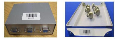
When a batch of individually tagged work-in-process is to be tracked, the process starts out by printing out the barcode/RFID tags, one for each item to be tracked. This also results in an entry for each item being created in the containers table in the BellHawk, which is associated with the work order and/or customer order for which these items are intended.
