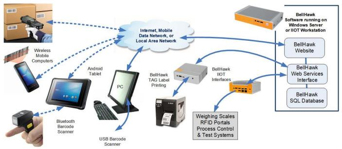
The BellHawk software can be run on a Windows Server computer or a Windows IIOT (Industrial Interface of Things) computer. It consists of a specialized web-server, with a web-services interface, and a SQL Server database.
